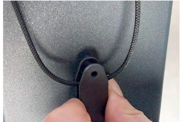
6.) Mounting spring tensioner: Apply tension to the cord, define position.
