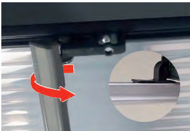
14.) Attach the velcro® profiles. Please note that the connecting hooks fixed with screws are always mounted on one side and the moveable hooks all on the opposite side of the longitudinal profile.
