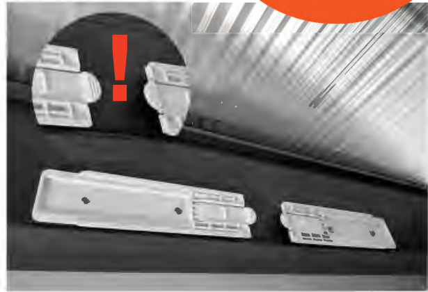
7.2) Attach brackets to the cross profile in the direction shown. Distance to the side rails 200 mm. The distance between the motors varies.
