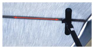
**3.** After attaching the fabric, press it along all velcro<sup>®</sup> strips once again with help of the operating rod!
